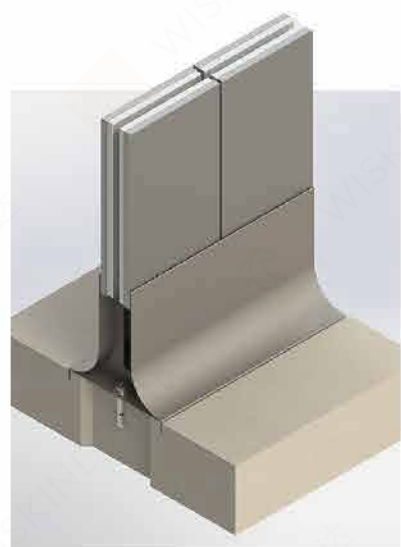
01. Waterproof wall base with stainless steel panel
