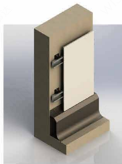
05. Waterproof wall base with hanging panel
