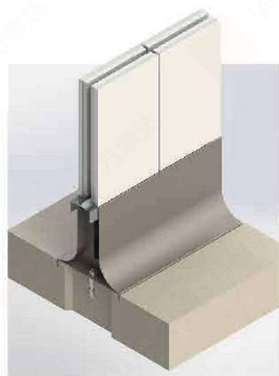
02. Waterproof wall base with color-coated panel
